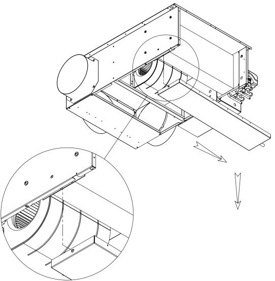
• Allow the rear end of the pan to drop slightly and pull the pan towards the tail end until the screws in the sides of the pan clear the slots in the chassis side. Lower con pan.
